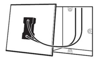
• Remove the clip cover and control plate from the switch mounting
