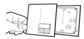
• Connect wires to the terminals of the dimmer
