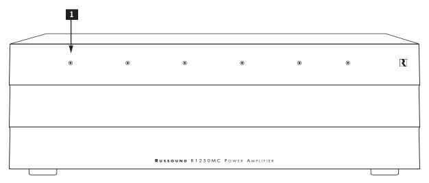
**1 Zone Indicator LEDs:** The six LEDs correspond to the six stereo zone amplifiers. The LED will illuminate red when the amplifier power is on and the zone is in standby. The LED will illuminate green when the zone is active.
