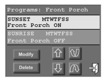
To modify or delete a program, highlight a program by simply touching the program in the list or by pressing the [up arrow] or [down arrow] buttons to scroll through programs. With each press, the next program is highlighted. Press the [page up] or [page down] buttons to scroll through groups of programs. With each press, the next group consisting of 2 programs is displayed, with the first program in the list highlighted.
