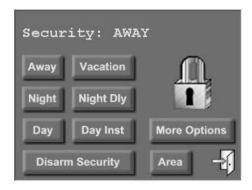
The top line on the "Security" page displays the current security mode.
