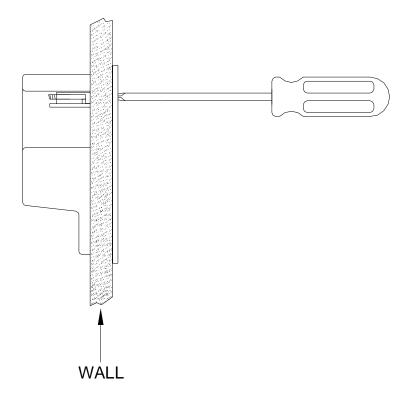
Before installing faceplate, remove the protective film from the LCD area of the touchscreen. Fasten the faceplate onto the touchscreen by hanging the top of the faceplate on the top edge of the touchscreen, then gently snapping the bottom onto the touchscreen.
