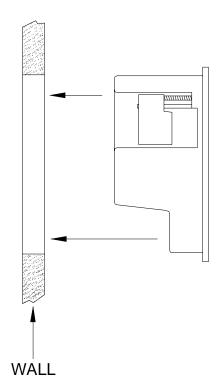
Place the assembled unit into cutout in the wall.
