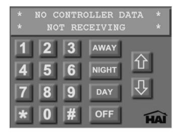
To assign an address to the OmniTouch touchscreen, press and hold the HAI logo for three seconds. The "Touchscreen Address" page is displayed.
