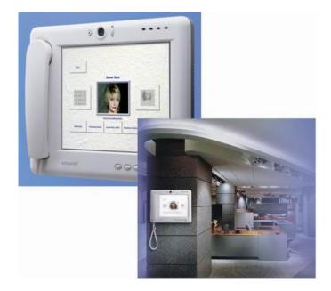
This product is an integrated system recognizing people by using multimodal biometric parameter. It has been designed and made for different uses. It used for access control, person presence tracking, time and attendance, controlling various devices and appliances etc. and also for sending and receiving video messages, for video surveillance and for video intercom.
