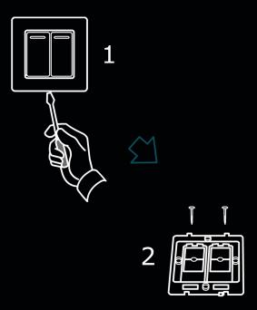
To open the cover by using the suitable tools. after connecting the wire, using the attached screw to fit the switch or socket on the line through the install eyelet.
