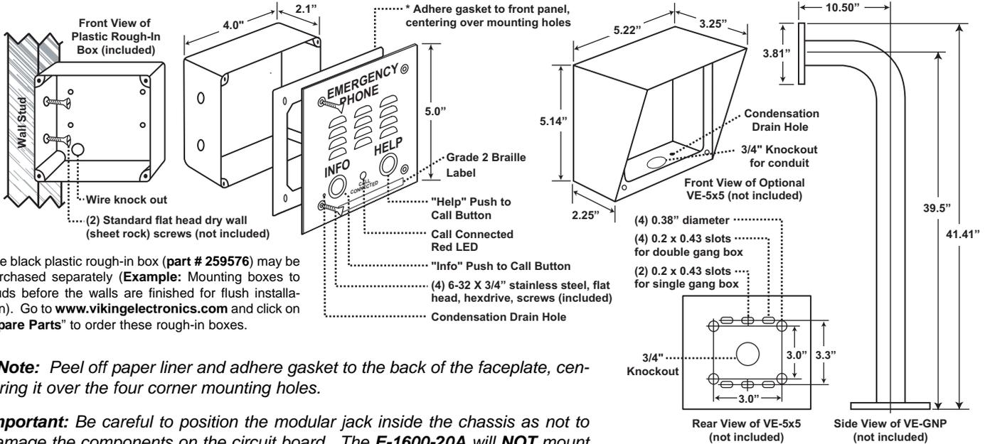
The black plastic rough-in box (part # 259576) may be purchased separately (Example: Mounting boxes to studs before the walls are finished for flush installation). Go to [www.vikingelectronics.com](http://www.vikingelectronics.com) and click on "Spare Parts" to order these rough-in boxes.
