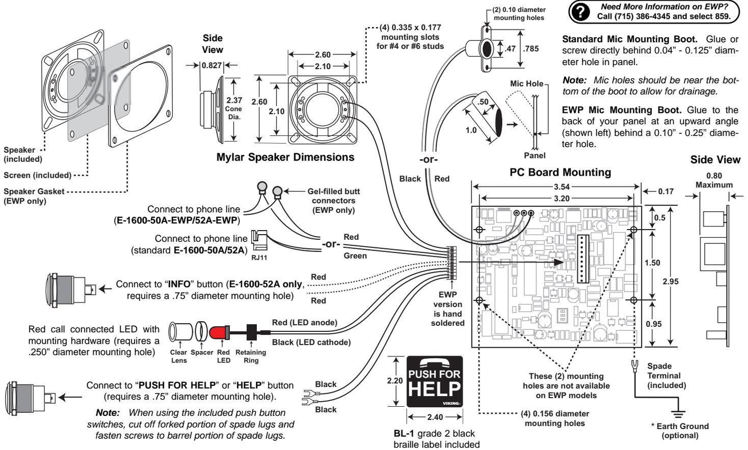
**Important:** If installing the EWP version outdoors, apply non-corrosive silicone (included with EWP version) to back side of LED and push button switches after making all connections and testing. Completely encapsulate exposed switch connections (screw terminals/stripped wires) and bare wire connections.
