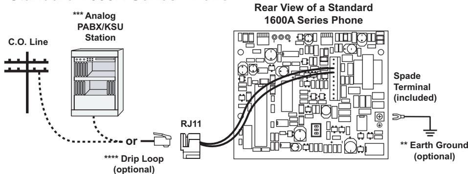
**IMPORTANT:** *Electronic devices are susceptible to lightning and power station electrical surges from both the AC outlet and the telephone line. It is recommended that a surge protector be installed to protect against such surges. Contact Panamax at (800) 472-5555 or Electronic Specialists Inc. at (800) 225-4876.*
