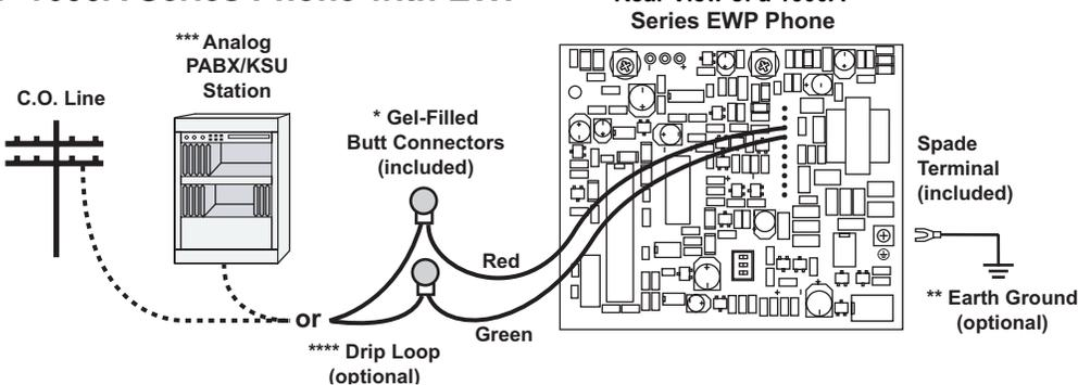
**\*\*\* Note:** *When installing a line powered phone on a low voltage and/or low loop current phone system extension, a PS-2R Talk Battery/Loop Current boosting power supply may be required. For more information on the PS-2R, retrieve Fax Back Documents 512.*
