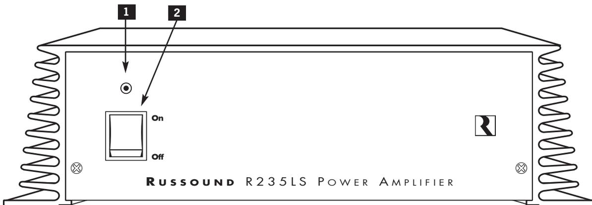
**1 Power LED:** The LED will illuminate red when the power is on and the amplifier is in Default/standby mode and illuminate green when the amplifier is active.
