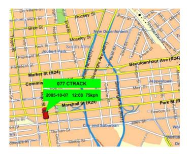
C-track Solo is based on a newly developed hardware platform utilising the Global Positioning System (GPS) to provide vehicle position to within 10 metres average accuracy and the GSM (MTN, VODACOM & Cell C) networks to transmit information real time 24-hours a day, all year round. This information can be sent directly to the customers base station, or first processed by the DigiCore Information Bureau to provide the customers with useful information to manage his fleet optimally.
