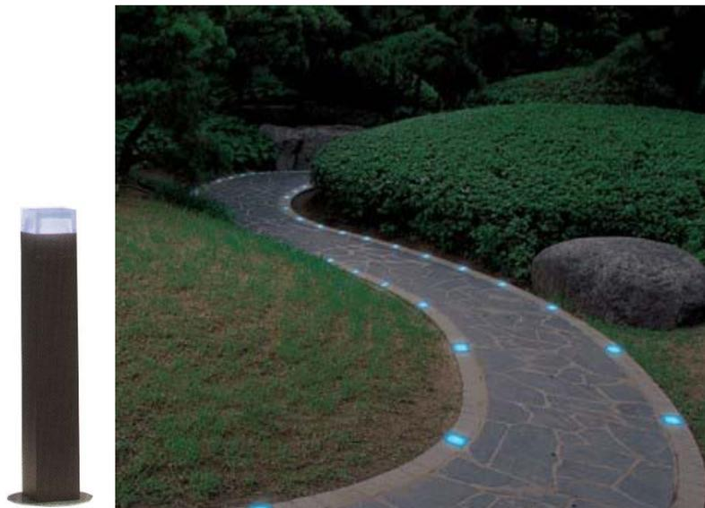
Recessed cube-shaped paver with high luminous intensity. Tempered glass body with frosted slip-proof finish. The base is made of stainless steel. Powered with LEDs (50,000 to 100,000h average lamp life) with stabilizing electronics for even luminous output. It is available with white, blue, red, green or amber light. Operates at 12v using standard light transformers and a power consumption of approx 1w. Two light tone combinations can be produced to special order.
