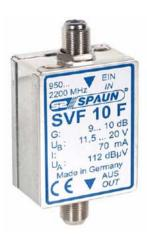
SAT-IF Amplifier is an integrated high-pass filter suppresses undesirable LNB intermodulation products in the frequency range below 950 MHz and this is for distribution of SAT-IF only this product is All DC through paths are both 22kHz tone (DirecTV) and DiSEqC (Dish Network) compatible and has a Remote powered by satellite receiver
