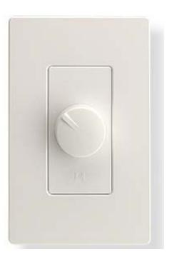
ALTx-2D UltraMatch<sup>™</sup> Volume Control with Decora® insert and Cover Plate, it is a wall-mounted, Decora® style, speaker-level, UltraMatch<sup>™</sup> volume control. It connects between the speaker outputs of an amplifier or receiver and a pair of speakers. The 1x setting allows the volume control to be used as a standard non-impedance matching control. The 2x, 4x, and 8x settings allow it to be used as an UltraMatch<sup>™</sup> control.
