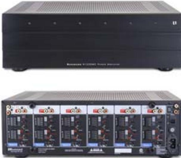
The R1250MC is a 12-channel power amplifier ideal for use as the main amplifier in home theater and distributed audio systems. The 12 channels are arranged in pairs to provide amplification for six stereo zones. The R1250MC provides an array of useful features such as bridged mono operation, independent zone triggering, bus inputs and multiple speaker outputs per zone to meet a wide variety of applications and configurations.
