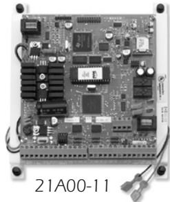
Omni LT Board Only 21A00-2 Omni LT controller board only.
